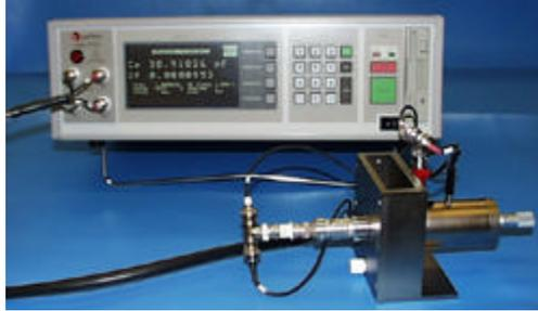
Figure 31: QuadTech 7000 Meter with LD-3 Cell
