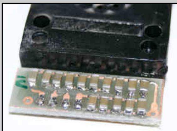
A small PCB with fifteen 1206-size ceramic caps fitted neatly on the back of the switches I used.
